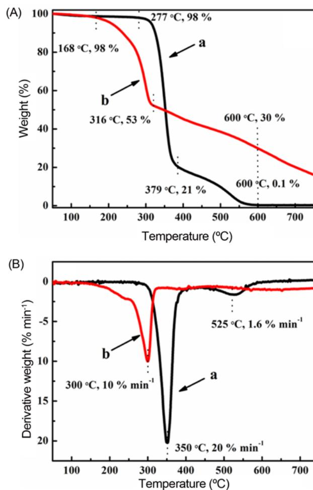
**Figure 2.** (A) TGA and (B) DTG curves of cotton fabric with and without finished treatment, (a) pure cotton fabric and (b) cotton fabric treated with optimal combination.
