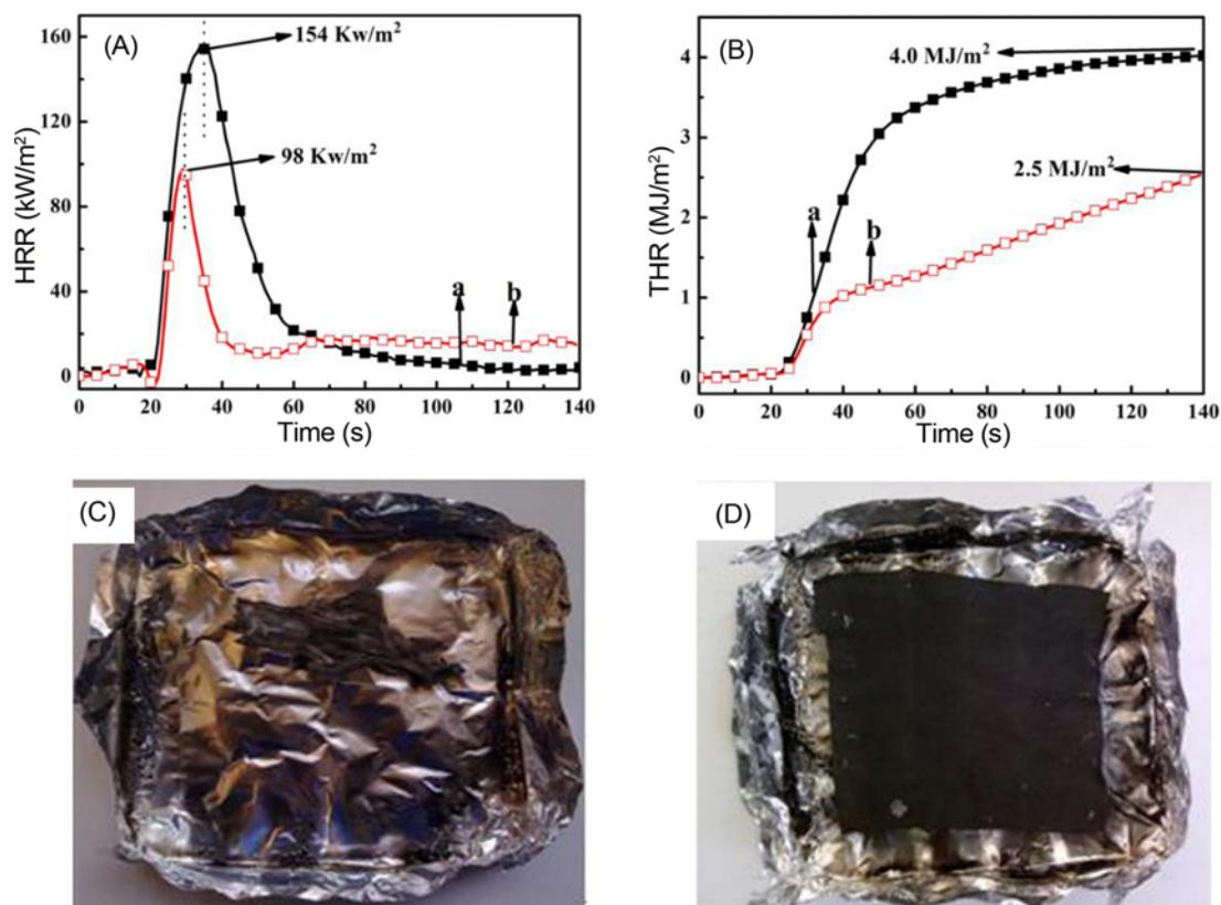
**Figure 3.** (A) Heat release rate curves, (B) total heat release curves of (a) pure cotton fabric and (b) cotton fabric finished with optimal combination, (C), (D) digital photos of the residues after cone calorimeter test for pure cotton fabric and the cotton fabric finished with optimal combination, respectively.
