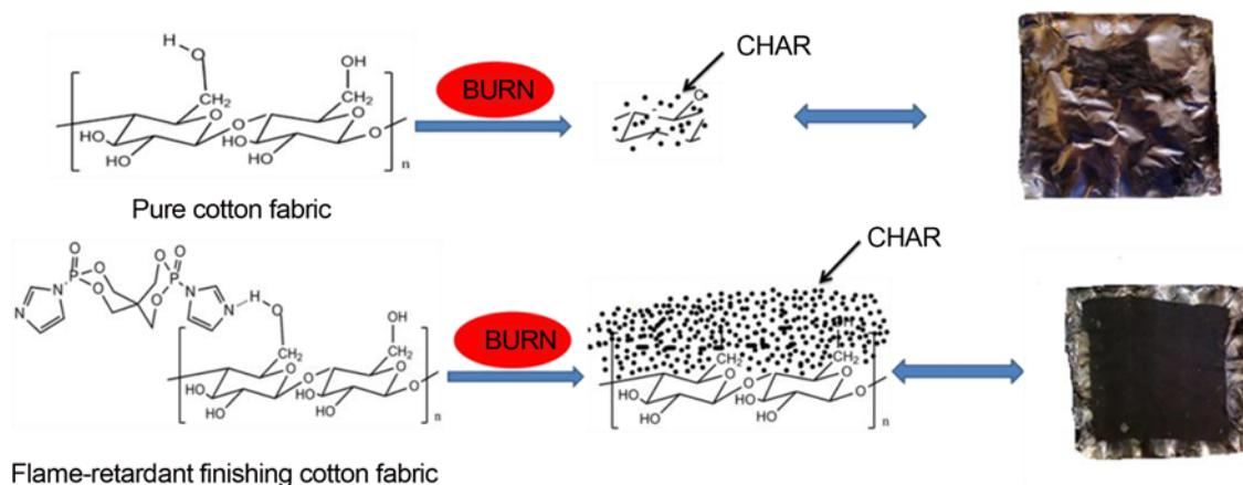
**Figure 4.** Schematic of the char formation.
