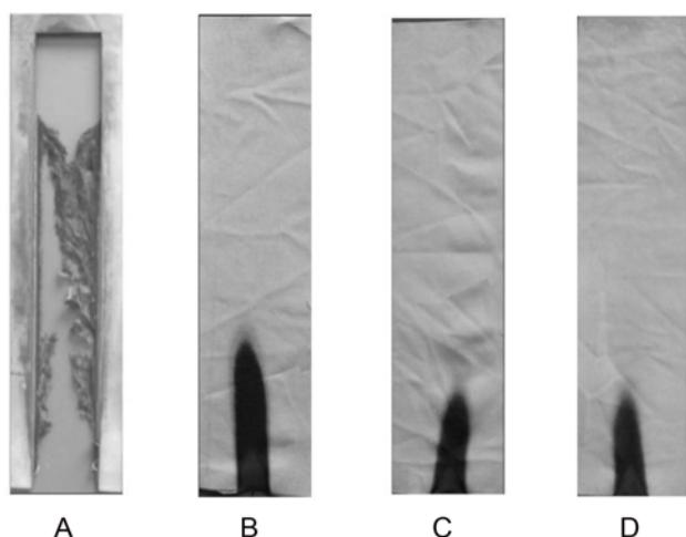
**Figure 1.** The damaged length after vertical flame test of (A) pure cotton fabric, (B) the 3th treatment, (C) the 24th treatment, and (D) the cotton fabric finished with an optimal combination treatment.
